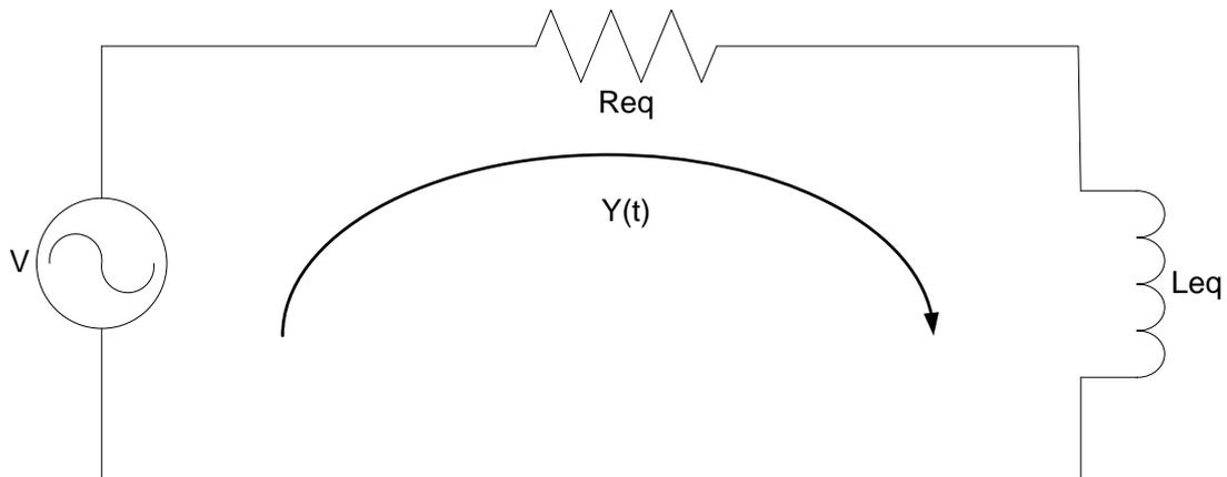
**Figure 3:** Equivalent circuit diagram of the model
